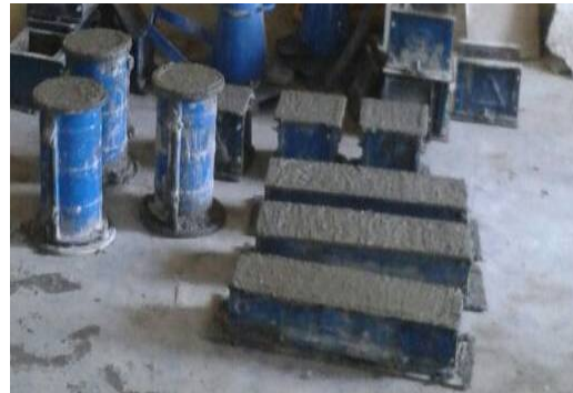
Fig.2 Concrete cubes casted in moulds
